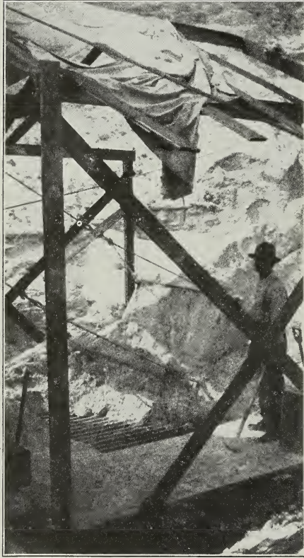
Fig. 35. Drag-line scraper bringing sand on to bar grizzly. (Photograph by courtesy of American Silica Sand Company.)
